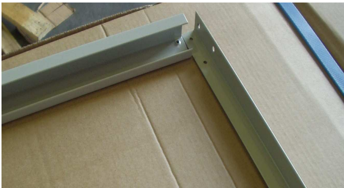
STEP 3: ASSEMBLE THE FIX END OF THE SHORT MEMBER WITH LONG MEMBER USING SCREW
